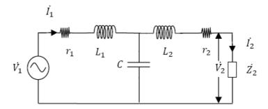
Fig. 2.3 T-LCL type immittance circuit
