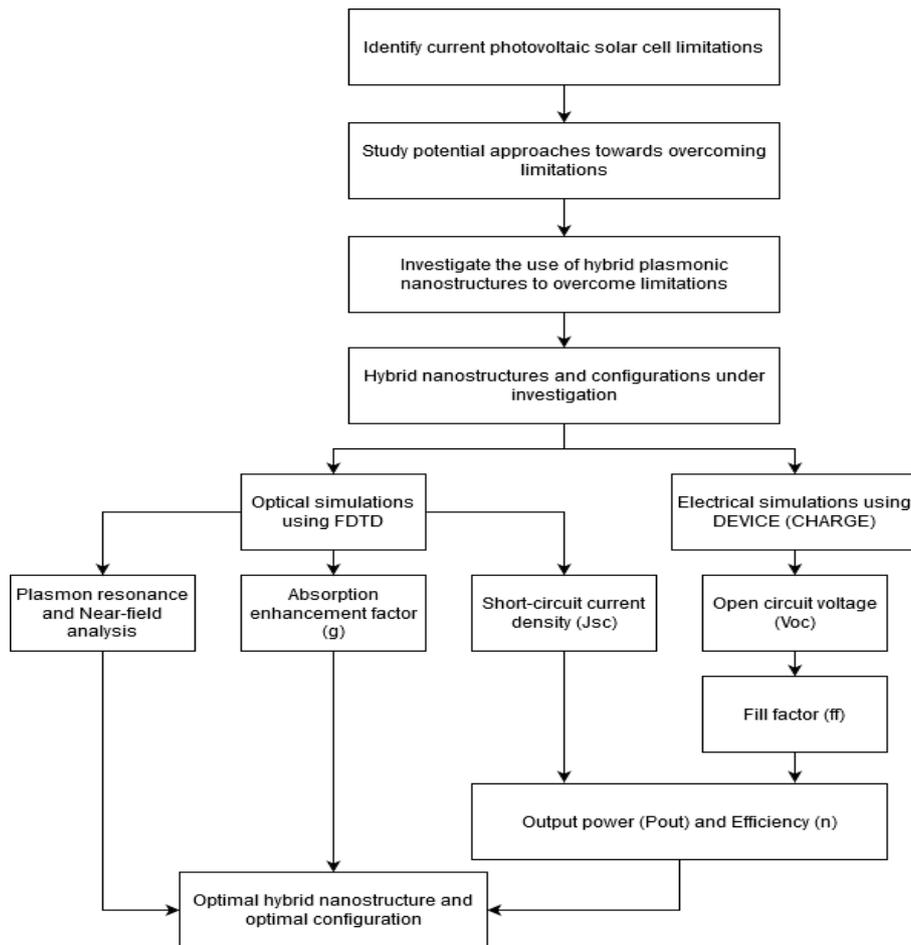
Figure. 2. Flow chart showing the steps that will lead towards establishing an optimal hybrid nanostructure design to aid in increasing the opto-electronic performance of thin-film solar cells.
