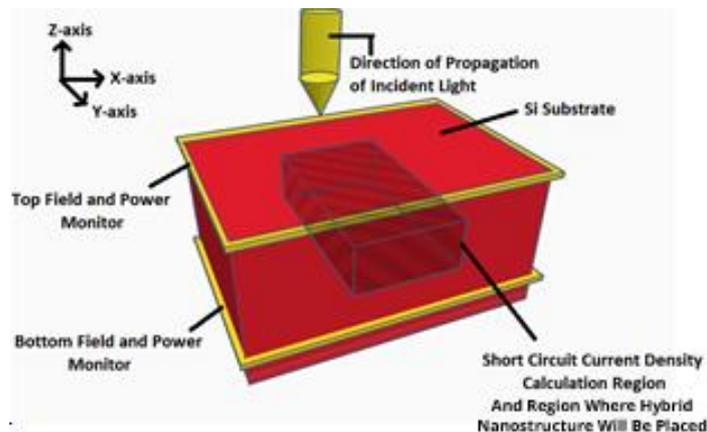
Figure. 3. FDTD Simulation setup for optical absorption enhancement ( $g$ ) analysis, utilizing frequency domain field and power monitors.
