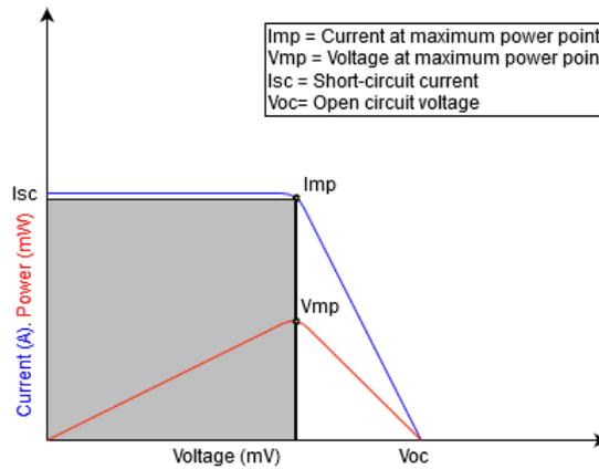
Figure. 4. I-V and P-V curves of a photovoltaic cell [37].
